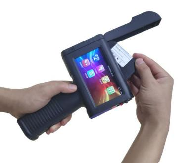
Bentsai's unique hardware protection scheme can disassemble and install the ink cartridges when the machine is turned on, without worrying about damaging the print head, giving you a different experience.
