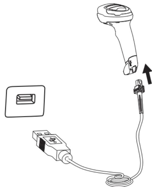
Connect the scanner to a Host through a USB cable with RJ45 and USB connectors:
