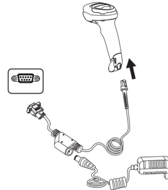
Connect the scanner to a Host through an RS-232 cable with RJ45 and RS-232 connectors and a power jack:
