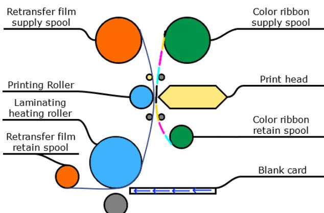
Retransfer print technology is the next level up to Direct-to-Card print technology. First, the image is printed on a film, then the image is transferred from the film to the card. This technique is suitable for Over the Edge, heavy duty printing, improves reliability and is suitable for a large variety of card types, such as:
